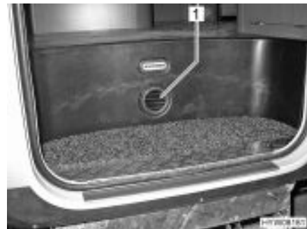
Fig. 88 Intake opening on the inlet shaft
