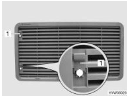
Fig. 98 Refrigerator ventilation grill (with sliding trap)
