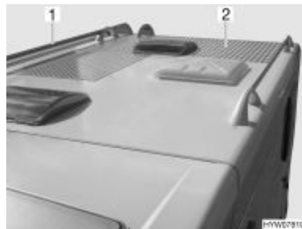
Fig. 1 Roof rail and step
