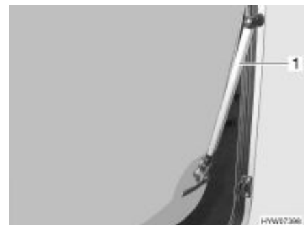
Fig. 38 Hinged window with automatic hinges
