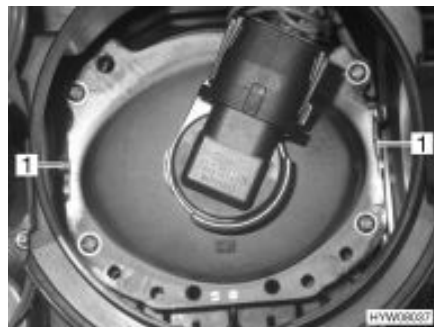
Fig. 126 Adjusting front headlight
