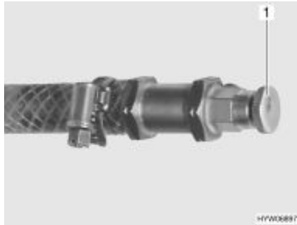
Fig. 120 Bleeding valve of hot-water heater
